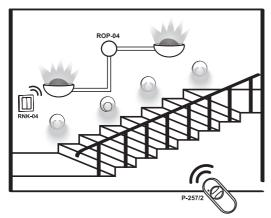
Wall lamps and standard LEDIX series LED fittings are connected to the ROP-04 receiver. 4-channel button radio transmitter RNK-04 and a portable remote control P-257/4 cooperate with the receiver. The wall lamps are switched on in time mode (staircase function) and LEDIX fittings in the switch on / switch of mode.
